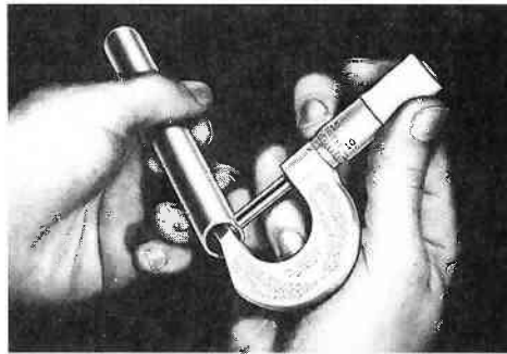
(c) Measuring tubing wall thickness with a round anvil micrometer
