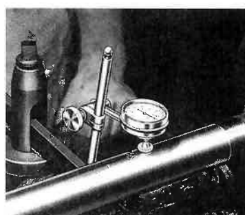
(d) Lathe operator uses dial indicator to check total indicator runout (TIR).
