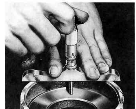
(f) Measuring the depth of a shoulder with a micrometer depth gauge
