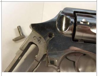
While holding the trigger back, pull the hammer free.
