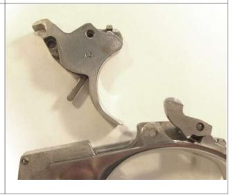
Remove the trigger plunger [47] from the trigger.
