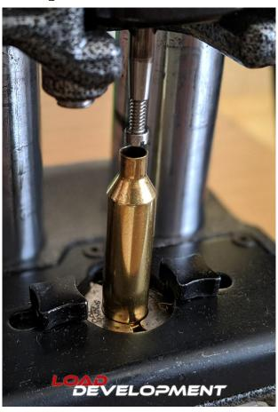
Because the neck expander ball is removed from the full length sizing die or if using a body die, it does not have a expander ball, the necks then still have to be expanded or sized up to the correct size for the bullets to be able to fit into them, and be seated. The reason we do not prefer using expanding balls that come with the FL-sizing dies, is because they often do not track perfectly straight when pulling them out, causing your necks to not be sized perfectly straight or symmetrical.
