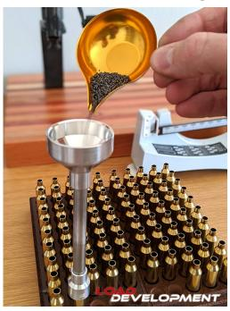
You then gently hold your funnel tightly on your casing, ensuring there are no gaps between the funnel and the neck of the casing, and then pour your powder through the funnel into the casing. Make sure all the gunpowder passes down the funnel into the case, and that there is no gunpowder stuck to the sides of the funnel. <u>Aluminum reloading funnels</u> tend to suffer less from static electricity build up and cling, than plastic funnels.
