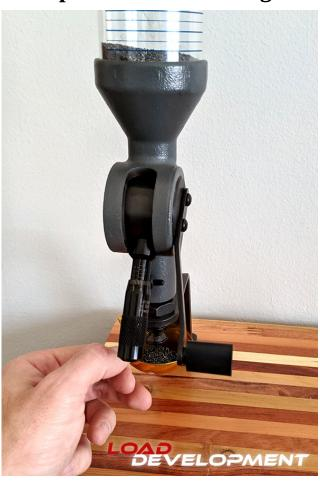
There are a few different ways how to measure powder for reloading, either with a <u>auto dispenser</u>, <u>auto trickler</u> or normal <u>powder dispenser</u>. Most manual powder dispensers have a micrometer on them, so you can set the amount of gunpowder it should dispense with each pull of the lever.
