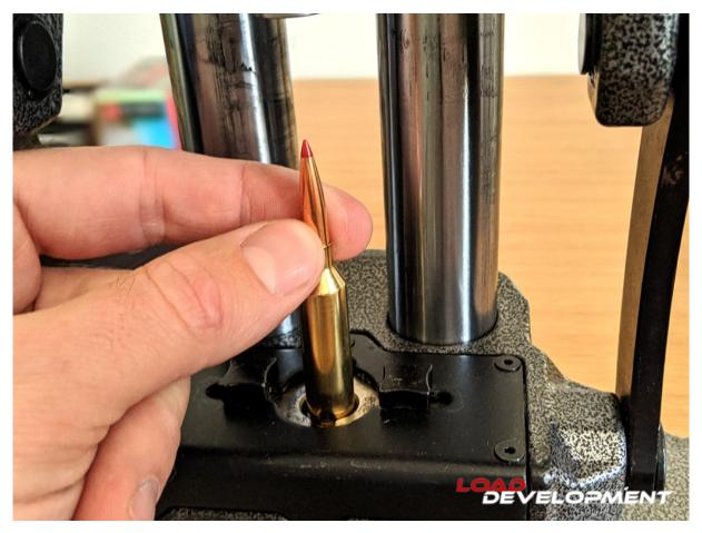
Place the case with powder charge into the shell holder of the reloading press, and then place a bullet into the casing.
