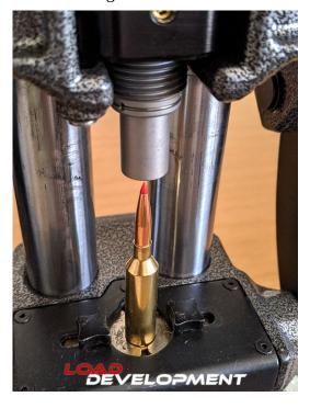
Making sure the bullet stays fairly straight, pull the lever on the reloading press, to lower the seating die onto the bullet, and press the bullet into the casing. Then lift up the lever again halfway, just so the seating die is off the bullet, rotate the bullet 180 degrees, and press it down again, just to ensure concentric bullet seating (maybe overkill with modern single stage reloading presses, but it just gives me piece of mind for accurate reloading).
