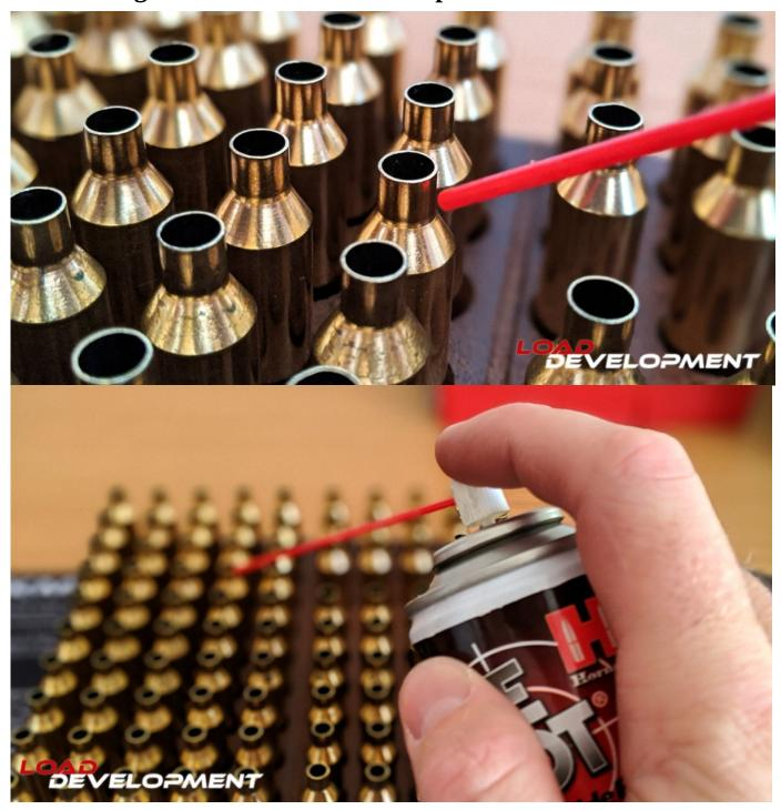
Thoroughly lubricate the necks of your casings with suitable <u>case lube</u> (lots of seasoned reloaders and precision rifle shooters do not recommend the Hornady One Shot case lube, and rather prefer <u>Imperial Sizing Die Wax</u>, but both work fine for me, the Hornady One shot just takes more effort on the press handle), making sure not to spray it inside the casings. If you use enough case lube on each casing, the effort needed to resize them, or bump the shoulders back, will be less.
