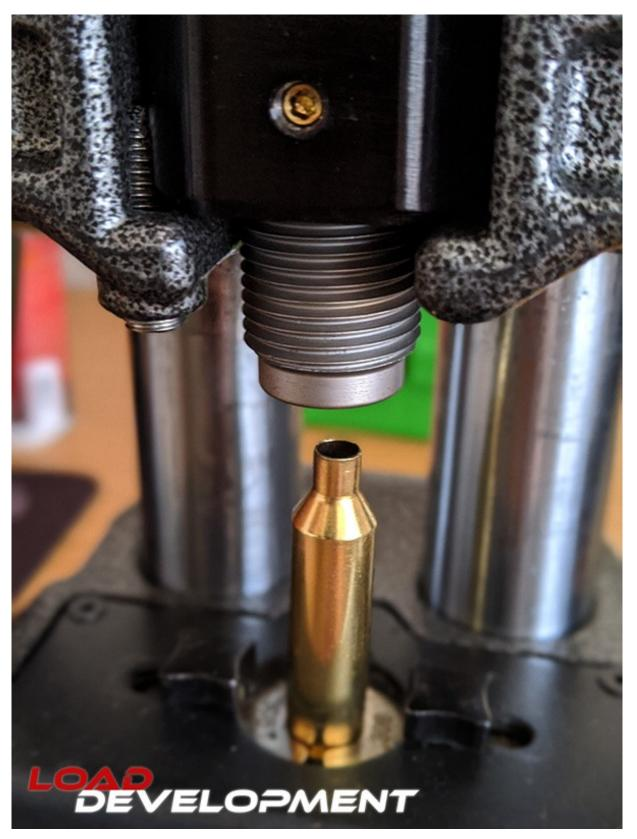
Now place the case into the shell holder on the reloading press, and pull the lever to press the full-length resizing die down onto and over the casing. Some people prefer to fully resize the casings after each fire, some after ever second or third fire, depending on how hard it is to close your rifle action when the cartridge is inserted into it.
