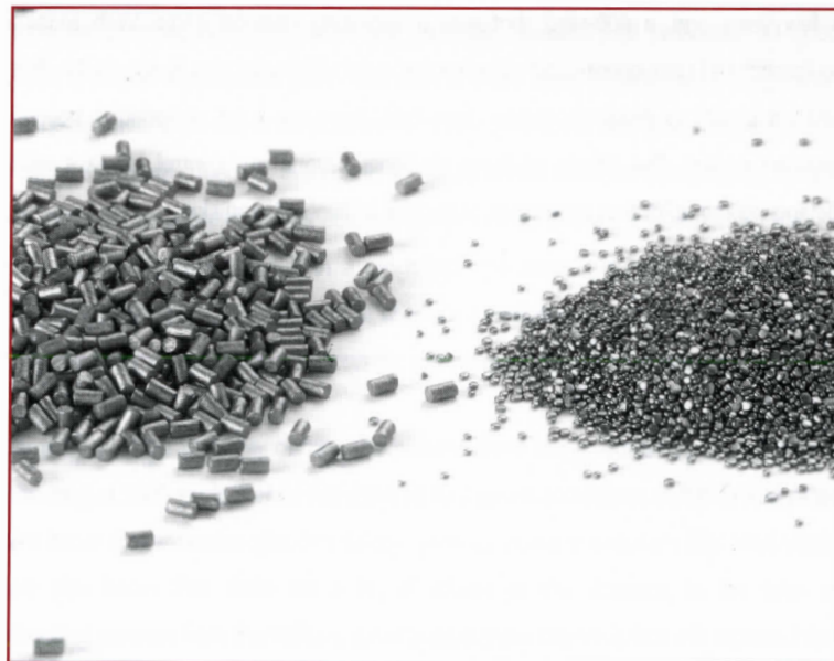
Propellants for rifle cartridges are primarily extruded, left, and spherical. If you look closely at the granules, you can see the reasons for the designations.
