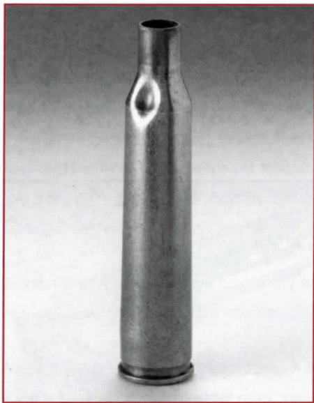
If you apply too much lubricant to the case, the lubricant will pocket at the shoulder during sizing and produce a dent, as shown here.
