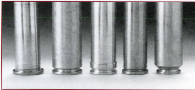
These represent various types of cartridge rim designs. From left are the rimmed, rimless, belted, semi-rimmed, and rebated.
