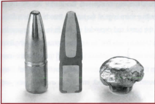
The Swift™ A-Frame™ bullet has a front core that is bonded to the jacket for ideal mushrooming and high weight retention.
