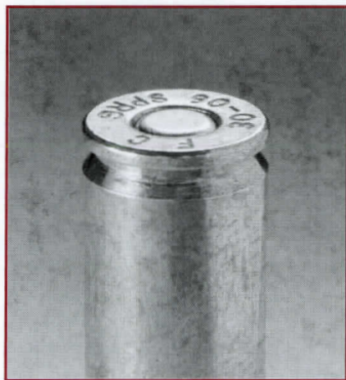
Primers should be seated flush with or slightly below the case rim. A primer should not project from the base of the case.
