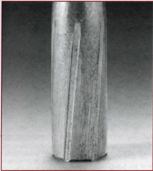
The idea of making a bullet spin during firing was a great improvement. Helical grooves can be seen on this bullet. The grooves were made by corresponding rifling in a barrel.
