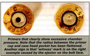
For safety's sake, always assume the hard bolt opening is signaling excessive pressure. However, having difficulty opening the bolt could also be due to a mechanical problem with the rifle such as a rough or dirty chamber.
