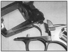
**REMOVE MAINSPRING.** Remove the mainspring (and your retaining pin, nail, or punch) as a complete assembly. **DISSASSEMBLY should only be performed if it is in need of repair or replacement.**
