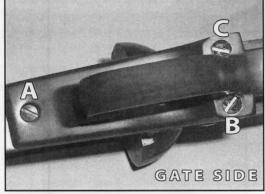
**5 SEPARATE GRIP AND CYLINDER FRAME.** Slowly, pull the GRIP FRAME towards the rear and down to separate it from the CYLINDER FRAME. Cocking the hammer back about a 1/4 inch may help in separating the two frames.
