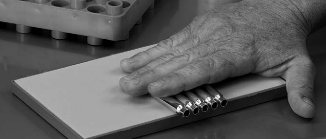
Roll cases on an RCBS Case Lube Pad for proper lubrication.
