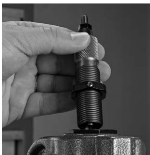
Screw Sizer Die into press.
