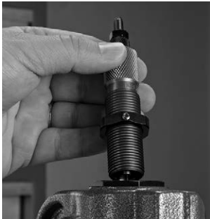
Screw Sizer Die into press.
