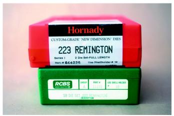
Choosing a suitable sizing die will help assure proper chambering of loaded rounds. The Hornady .223 Remington dies are "full length" making them suitable for most bolt actions, etc., while the RCBS "small base" dies are best for autoloading, pump and lever-action rifles.
