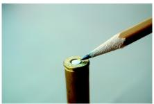
Proper priming will assure reliable ignition. Most companies recommend primers to be seated .003 to .005 inch below flush, allowing the anvil to be in contact with the bottom of the primer pocket. tolerance changes can cause pressures to spike in a given gun, while the same load was safe in the test gun or pressure barrel. Excess headspace, an out-of-spec firing pin or firing pin hole and other issues can cause a primer to rupture. Again, don't start with maximum loads.
