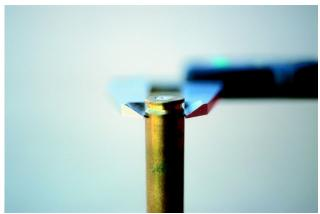
Case head expansion should be checked using calipers that are capable of measuring 0.0001 inch. High-pressure rifle cartridges usually expand .0003 to .0005 inch and are generally considered to be around 50,000 CUP.
