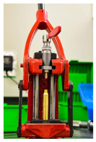
A bullet puller is an important tool for reloading. It will enable you to easily pull bullets and disassemble loads that you don't need to test. This is a collet type bullet puller made by Hornady. It retails for about \$25 and caliber-specific collets are about \$10 each. Pulled bullets can be re-shot, but I typically save them for fouling rounds.
