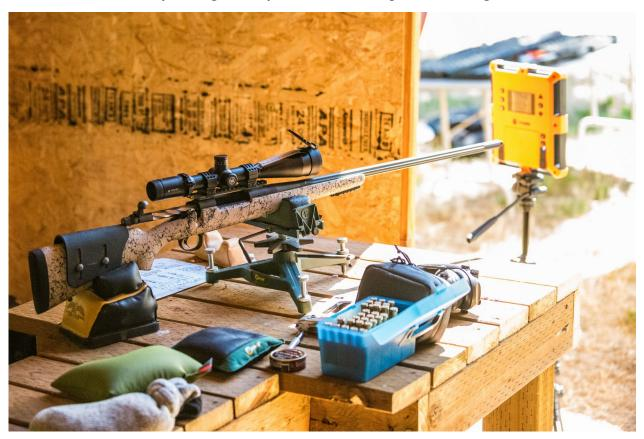
Tracking velocities during load development can help you spot high pressures before you see the damaging signs on your brass.
