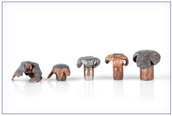
There are three main types of expanding jacketed bullets: hollowpoint (HP), soft point (SP), and partition. Within most of these types, there are features that improve performance such as polymer tips, boattails, etc. Many manufacturers have trademarked features meant to provide performance improvement. An example of this would be the Hornady InterLock.
