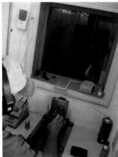
Image 4: Pressure laboratories use precisely made barrels that are likely to differ from the average factory barrel, resulting in different velocities with the same load.
