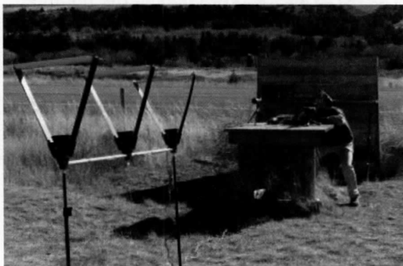
Image 1: Even a professional-grade chronograph, such as this Oehler, will give slightly varying readings depending on light conditions.
