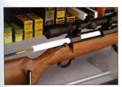
direction). Add CR-10 to brush while it's at muzzle end of barrel half way through process. Once the process is complete, clean the bronze brush with a blast of crudbuster or something similar.
