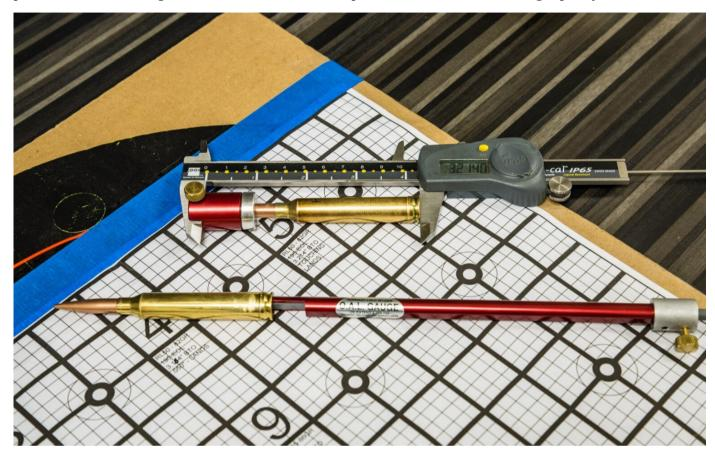
The Hornady OAL gauge and bullet comparator paired with a caliper will be some of your most valuable reloading tools.
