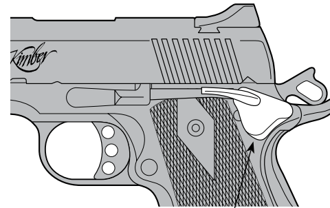
Thumb safety in "off" position
