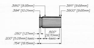
Cart. Case: Max. Case Length: 0.754" Speer Trim-to Length: 0.744" Primer: **CCI 500** Max Cart. OAL: Test Firearm: S&W M5906 1.169" **RCBS Shell Holder:** #16 Barrel Length: 4"
