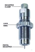
SCREW THE FULL LENGTH SIZER in until it touches the shell holder. Raise the ram; tighten the lock ring finger tight.
