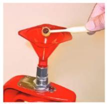
**CAUTION** After charging the case, the only operation that should be done is to seat the bullet. Never try to seat a primer after powder has been added.
