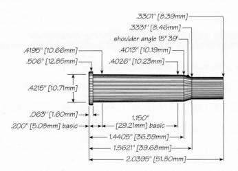
Max. Case Length: 2.0395" Cart. Case: Winchester Trim-to Length: 2.030" Primer: CCI 200: 250\* Winchester Model 94 Max Cart. OAL: 2.550" Test Firearm: **RCBS Shell Holder:** #2 Barrel Length: 20"
