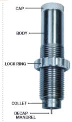
ADJUSTMENT FOR LEE PRESSES Screw sizing die in until it contacts the shell holder, plus one more turn (1% turns for Classic Series press owners).
