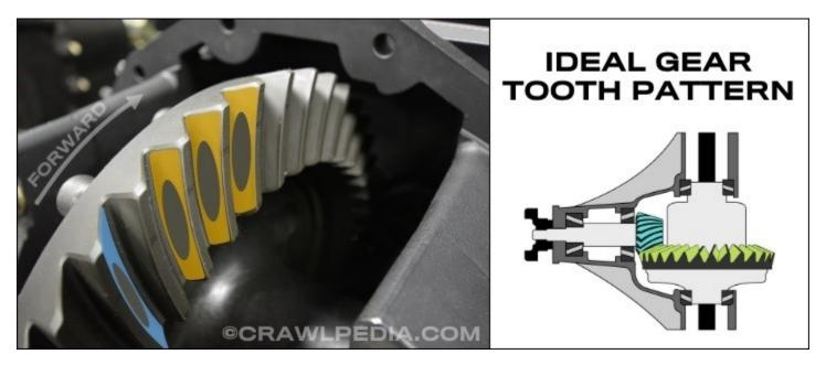
**The ideal gear tooth pattern** will have the contact patch on both the drive and coast sides of the teeth centered between the face and the flank as well as the toe and the heal. If your gear tooth pattern looks like the photo above, you have a perfect gear tooth pattern.
