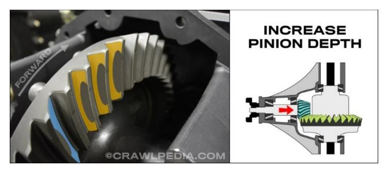
If your gear tooth pattern is too high, up towards the gear face, you will need to **increase your pinion depth** by using more or thicker pinion shims. This will move the drive side contact point down towards the gear flank (root) and slightly in towards the toe. The coast side contact pattern will also move down towards the flank but out slightly towards the heel of the ring gear.
