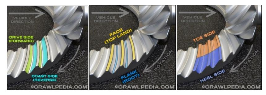
**Ring Gear** The large round gear that bolts to the differential. Also sometimes called the crown gear.
