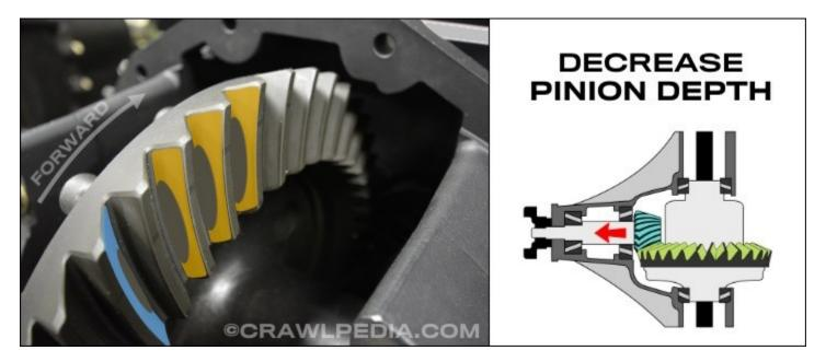
If your gear tooth pattern is too low, down towards the gear flank (root), you will need to **decrease your pinion depth** by using fewer or thinner pinion shims. This will move the drive side contact point up towards the gear face (top land) and slightly out towards the heel. The coast side contact pattern will also move up towards the face but in slightly towards the toe of the ring gear.
