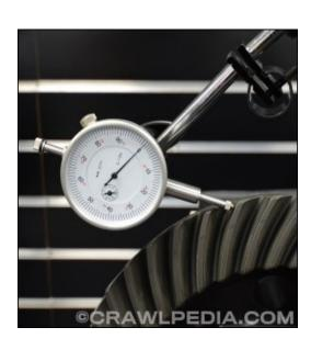
pinion yoke so it doesn't rotate. The distance that the ring gear moves is the backlash.
