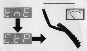
Turn the knob to "Full Throttle Position" (FtP). Hold the accelerator all the way down. Click the knob once, then double-click to set the current Full Throttle Position. Click again to exit.
