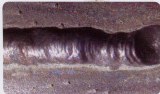
Weld Speed Too Slow
