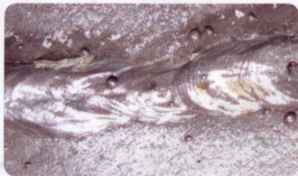
CTWD Too Long
