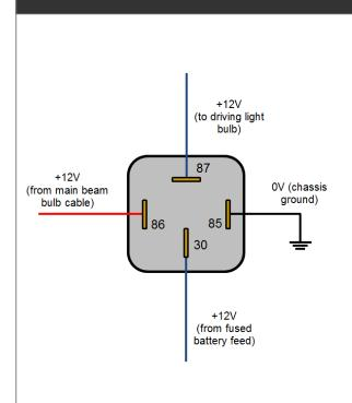
**Terminal 86** - Connect to the +12v cable feeding power to the headlight main beam bulb (achieved by making a splice in the original loom).
