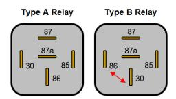
You will notice that on the Type B layout pins 86 and 30 are swapped over compared with the Type A layout. The Type B layout is arguably easier to work with as the connected terminals are in-line, making the wiring easier to visualise. If you need to replace a relay make sure you use one with the same terminal layout as it is easy to overlook if you're not aware of the difference.
